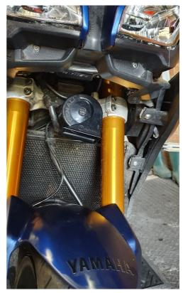
the bolt securing the original to the frame, remove the wires, put the wires to the sound bomb, fit the 2 brackets that come with the kit to the horn and then refix back to the frame. Simples! Ignition on and push the button. What a difference! Definitely louder but the tone is deeper as well.
