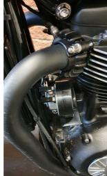
exhaust it was closer, so I just turned the horn around and fitted it the other way. The only thing I think I need to do is to get some black paint and give the facing side of the new horn a quick coat.
