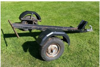
Built 20 years ago using plans contained in Classic Motorcycle Mechanics magazine, using new Indespension 350kg unbraked suspension units, with hubs to fit 10" Mini wheels.
