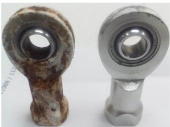
test they had done was a 72 hours environmental chamber salt corrosion test. The results were indisputable as shown in the attached photo. I think you can spot the difference. The test article is a rose end bearing from the gear lever mechanism.
