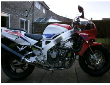
although I repaired them once with a bit of welding I finally gave in and bought some Motad stainless pipes.
